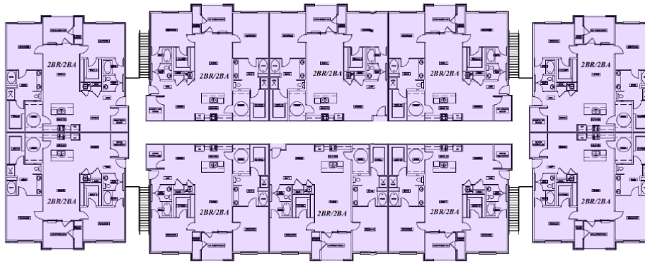
BUILDING 4 FLOOR PLAN - 3 STORY RESIDENTIAL 30 Residential Units
