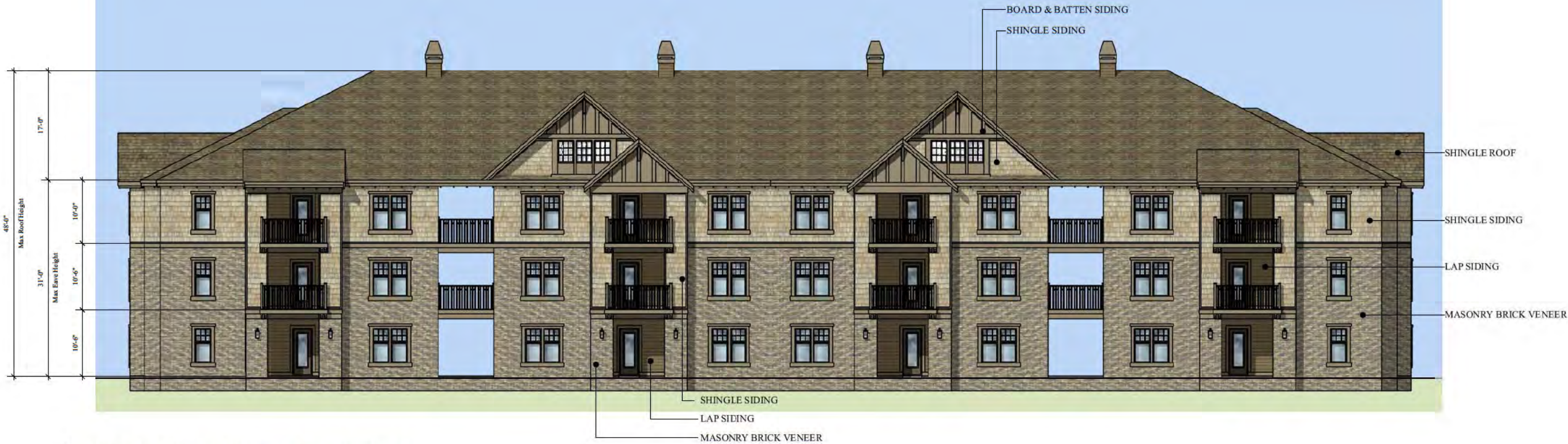
BUILDING 5 & 6 Concept Elevation - 3 Story Residential Residential Units (24 Unit - 2 Bed & 3 Bed) Scale: 1/8" = 1'-0"
