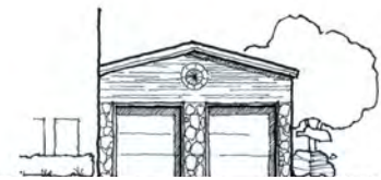
Figure 6-5. Only single entry doors are allowed if the garage is front loaded and facing the street.
