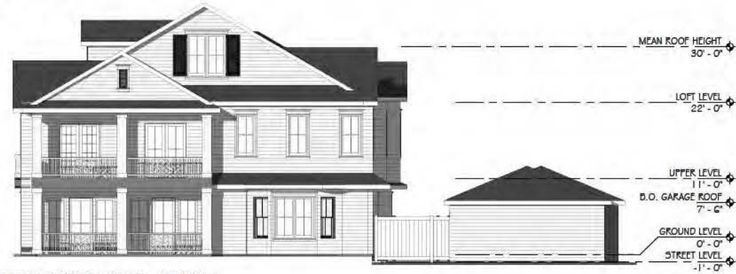
2 7 UNIT BUILDING - WEST SCALE: 1/8" = 1'-0"
