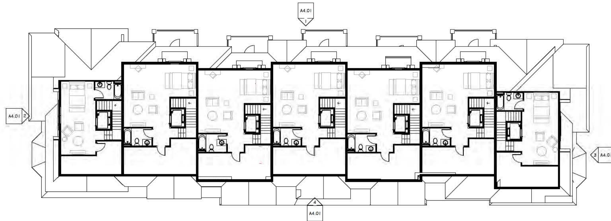
7 UNIT BUILDING - LOFT LEVEL SCALE: 1/8" = 1'-0"
