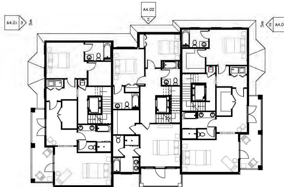
1 3 UNIT BUILDING - UPPER FLOOR SCALE: 1/8" = 1'-0"
