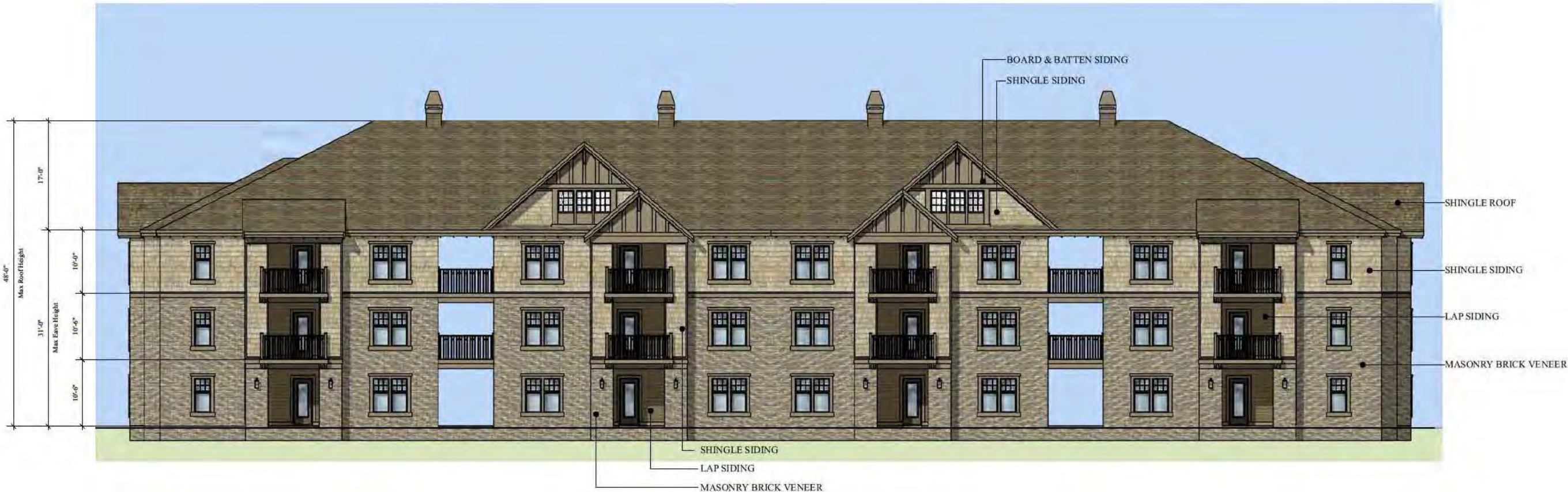
BUILDING 5 & 6 Concept Elevation - 3 Story Residential Residential Units (24 Unit - 2 Bed & 3 Bed) Scale: 1/8" = 1'-0"
